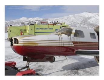
This Piper Malibu recently developed severe vibration, 'low oil pressure and a possible oil leak' several miles out from Aspen. The pilot managed to land despite an oil-coated windshield obscuring forward visibility. He later found the entire prop had 'departed' in flight
