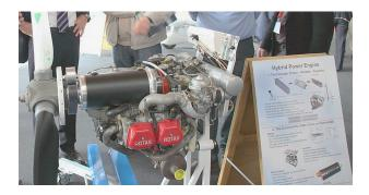
A standard Rotax 914 turbocharged engine is mated to a 40 hp electric motor and coupled to the propeller hub using a poly-V-belt drive. The basic Rotax, rated at 130 hp, together with the 40 hp electric motor, provide a combined 170 hp for takeoffs and climbs. This full power rating is available for a maximum 5-minute duration.
