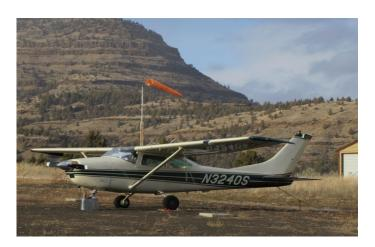
Answer: To keep the mice from climbing up the wheel and nose strut to nest in the cowling.
