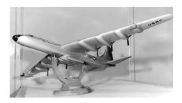
On paper the US plan was pretty simple. Place a 35-megawatt nuclear reactor in a modified B-36 and call it an X-6 or B-60. As the plane flies, it sucks in air, like a jet, and blows that air over the reactor core until it reaches 2,000F. Then blow that hot air into four modified GE XJ53 turbojets to create thrust. The modified XJ53 was called an X39.
