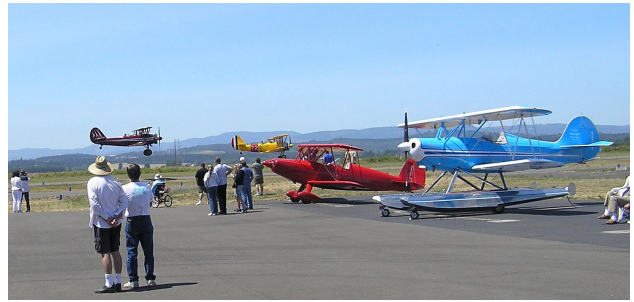
Two Waco's are taking off in the background. The pale blue airplane is a Hatz. To meet gross weight with floats, the second pilot seat access is blocked off.
