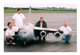
This C-17 Globemaster III is one of the largest jet models in the world today! Complete with retractable landing gear and pneumatically operated flaps. The four builders are shown above, with the model.
