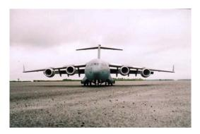
The model also has smoke systems both of the inboard turbines, and uses 2.4 GHz data link to provide real-time data to a laptop computer on the ground while in flight, this data includes airspeed, turbine RPM, EGT, fuel consumption, etc. It is covered in fiberglass and epoxy resin. Built mainly from balsa and ply, with many glass and carbon fiber moldings to reduce weight.
